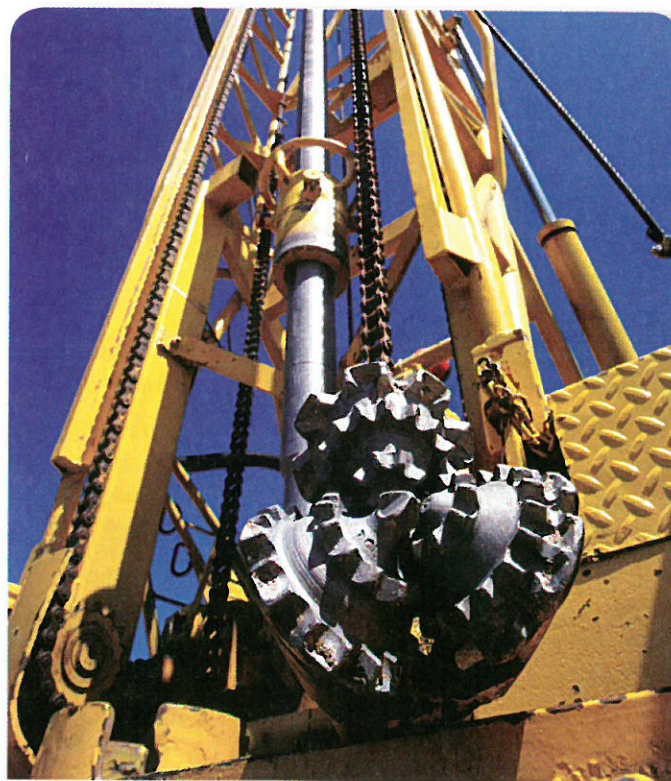
■ Figure 5.2 The temperature of Earth's upper crust increases with depth by about 30°C for each 1 km. At a depth of 3 km, this drill bit will encounter rock that is close to the temperature of boiling water.
